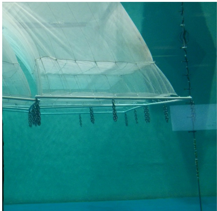
An experimental measurement of wake velocity downstream of a scale model square cage array, using 8 Swoffer current meters mounted to a vertical bar. The vertical bar was traversed across the flume tank to capture a plane of velocity measurements at certain distances downstream of the cages (photo credit: Adam Turner).
