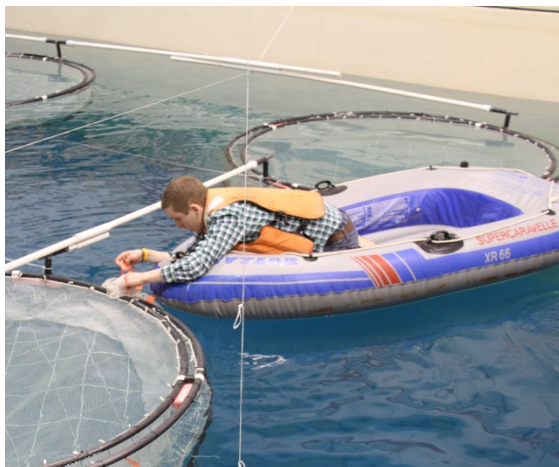
Adam Turner hard at work (and well dressed!) in the Supercaravelle XR66 dingy during the CIMTAN HQP workshop, attaching flagging tape to a scale model fish cage. Flagging tape was used as a method to visualize unsteadiness and turbulent structures in the wake of fish cages (photo credit: Justin Del Bel Belluz).
